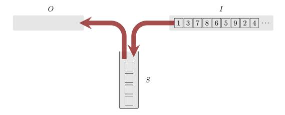
Remark: Comparisons are only possible between the element currently at the top of S and the element currently at the front of I. Hence between any two (non-redundant) comparisons we must have a move " $I \to S$ " or " $S \to O$ ".
